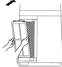
6. Install the air inlet grille Align the upper two buckles and press them tightly, then press the two sides at lower part, slowly and gently buckle the air inlet grille.
