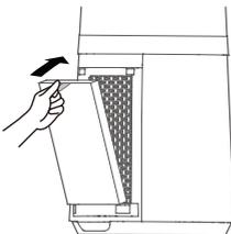
5. Install the pre-filter Align the slot position at the bottom, and buckle up the upper U-shaped buckle.
