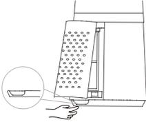
2. Take out the pre-filter Press the raised part on both sides to pull it outwards, and take out the pre-filter.
