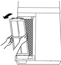
3. Remove the protective film of the filter.
